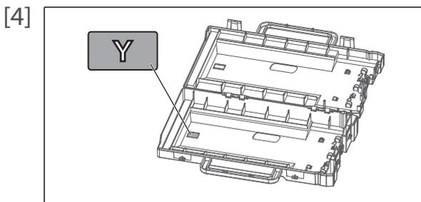
Open an ink case and apply an ink color label onto the inside of the case.
