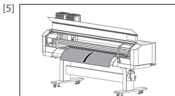
From the front side of the printer, pull the media for approximately 1 m.
