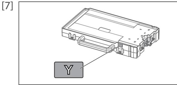
Apply an ink color label onto the outside of the case.
