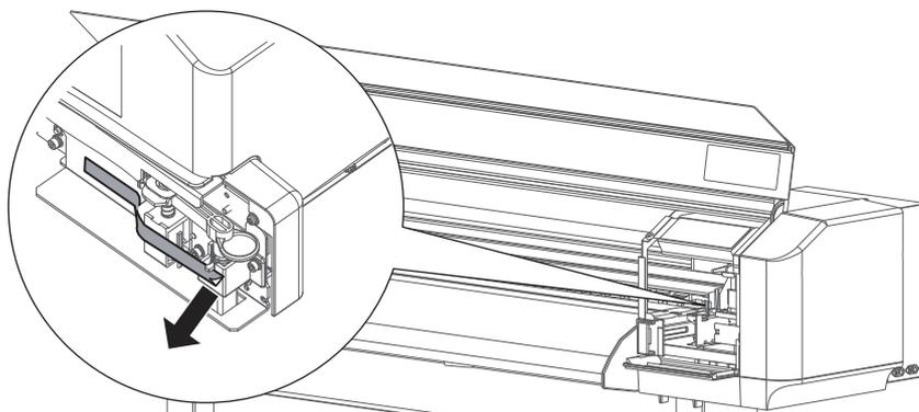
[6] Remove the wing bolt to remove the shipping bracket from the carriage.
