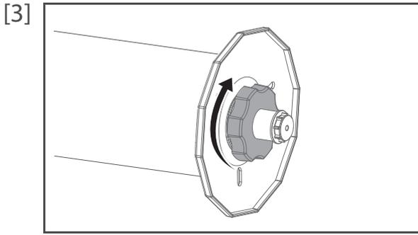
Twist the handle clockwise to lock the flange.
