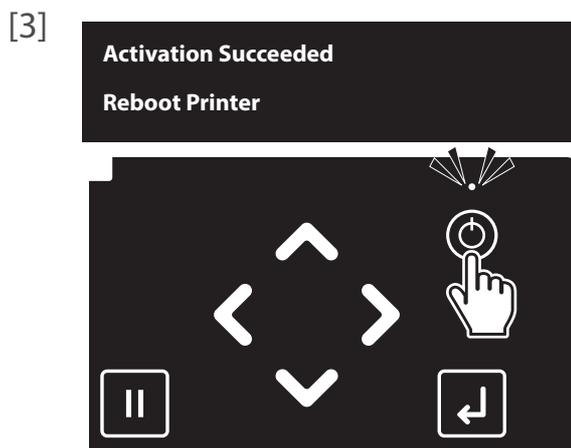
When the message on the left appears, long press the Power button to power off the printer.
