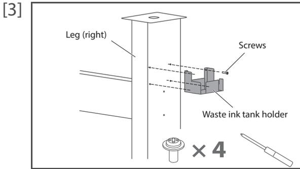
Use the round head screws (x4) to attach the waste ink tank holder to the right leg.
