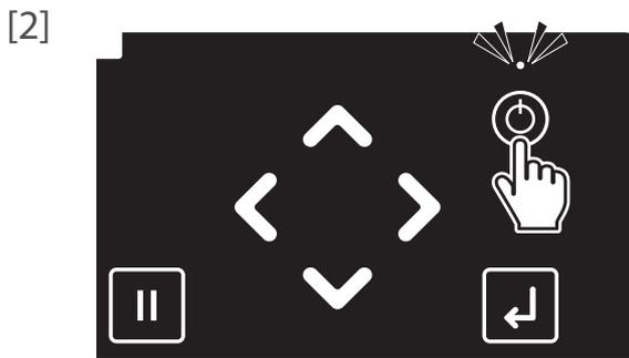
Long press the Power button on the front panel.
