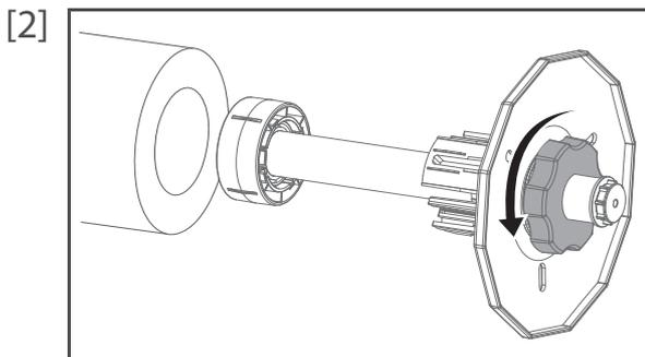
Push the media flange (x2) into the both ends of the media core.
