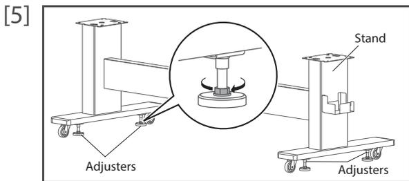
Turn the leveling adjusters (x4) as shown on the left until the stand does not move.
