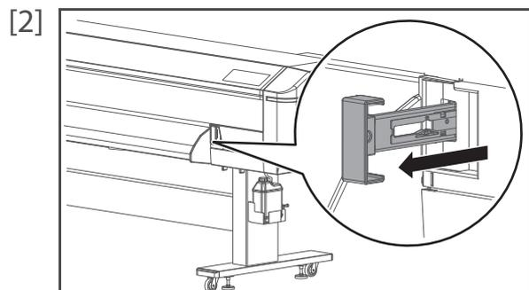
From the front side of the printer, fully pull the media feed lever towards you to release the pressure rollers.
