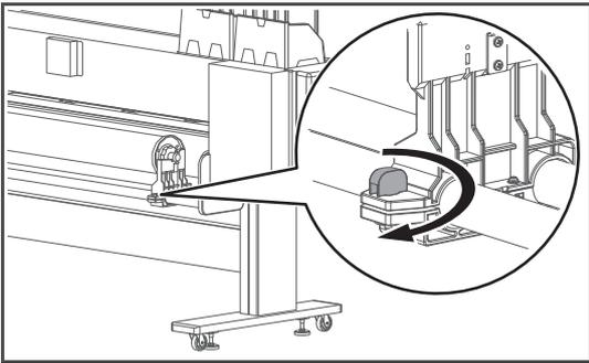
Twist the knob bolt on the right side of the media holder clockwise to tighten.
