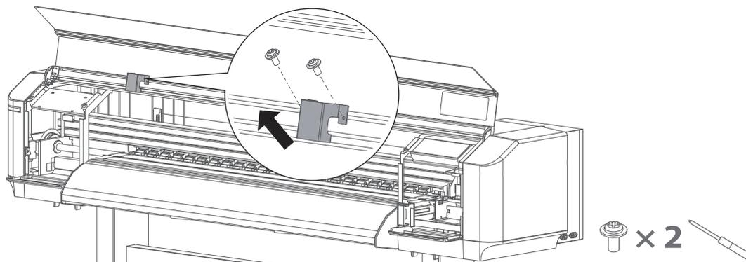
[4] Open the front cover and remove the protective tape from the maintenance cover.
